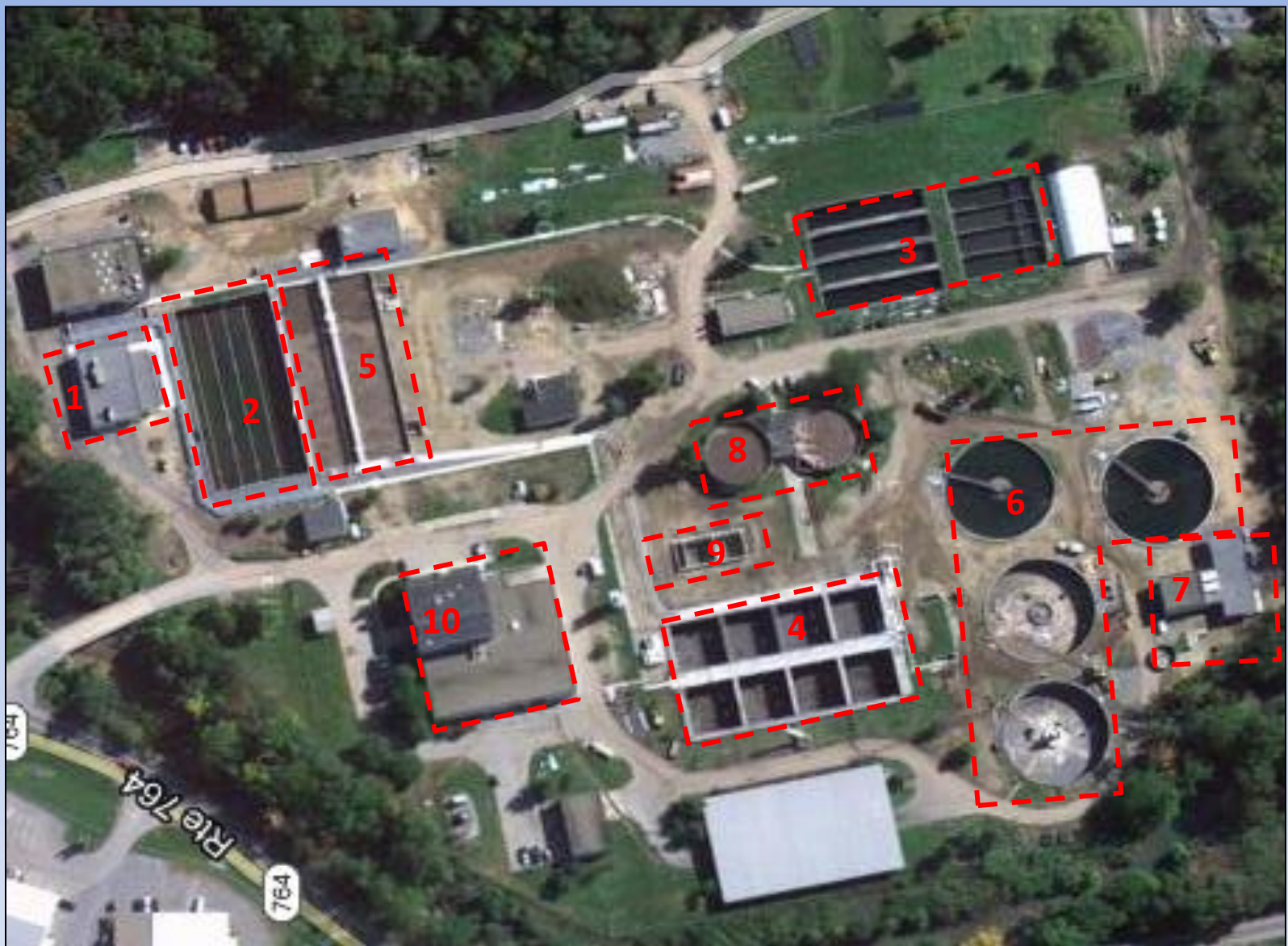
1) Headworks building, 2) Primary Equalization Tanks, 3) Secondary Equalization Tanks 4) BNR Reactors 1 & 2, 5) BNR Reactors 3 & 4, 6) Final Clarifiers, 7) UV Units, 8) Aerobic Digesters, 9) Digested Solids EQ/Feed Tank, 10) Control Building and Sludge Handling
